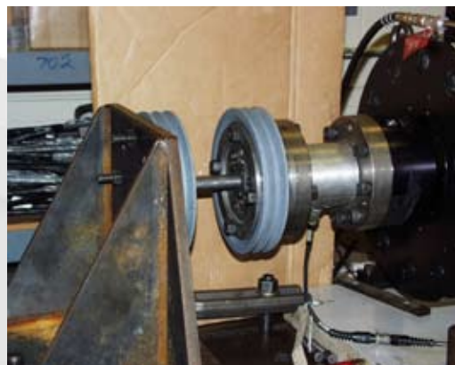
Reversing load torsional fatigue test using a hydraulic rotary actuator.
